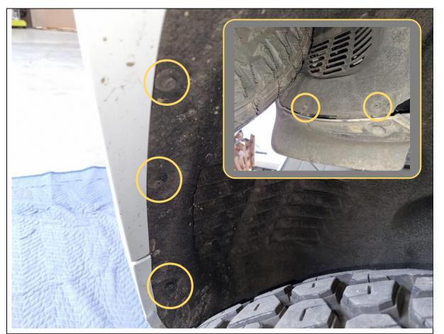
8. On each side, remove 5x 8mm hex head screws securing the wheel arch liner to the bumper.
