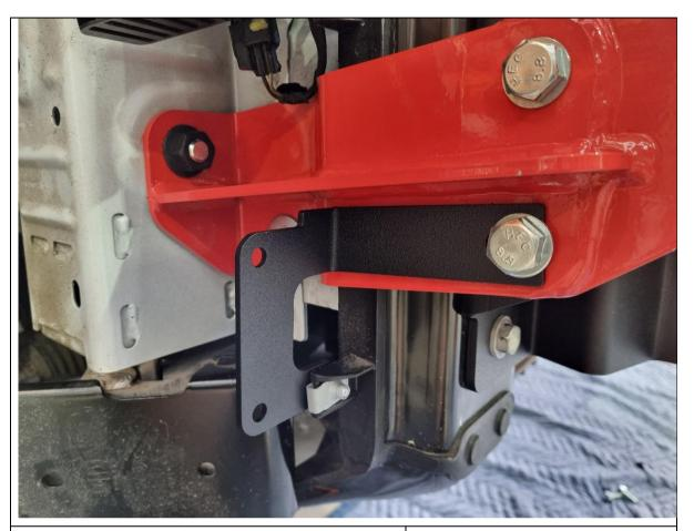
36. For 4xe owners, fit the supplied 4xe pedestrian alert speaker relocation bracket on the outside of the RHS recovery point and re-fit the speaker using the supplied M5 fasteners.
