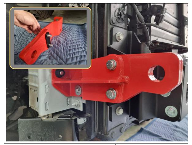
35. If fitting recovery points with Offroad Animal Hidden Winch, fit the recovery point to the hidden winch chassis mount with a P-0288 spacer plate (supplied with Hidden Winch kit, see inset) and the same M12x55 fasteners from Step 29.
