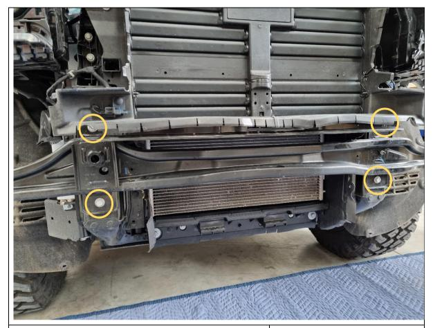
20. Using a 16mm socket or spanner, remove the 4x hex head bolts securing the impact beam to the body.
