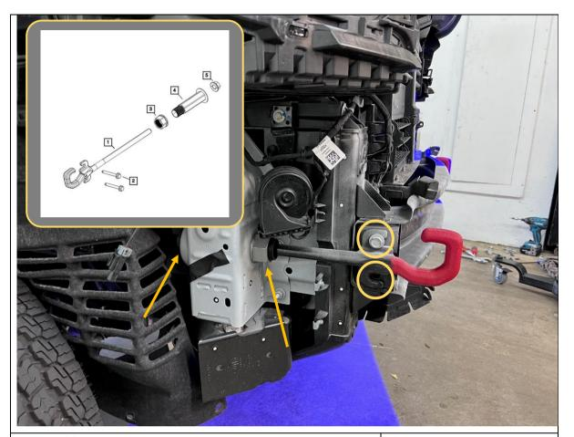
17. If factory tow hooks are equipped, remove them by undoing the 2x 16mm hex head bolts on each side, then remove the large nuts with a large adjustable wrench (see inset for Jeep parts breakdown).
