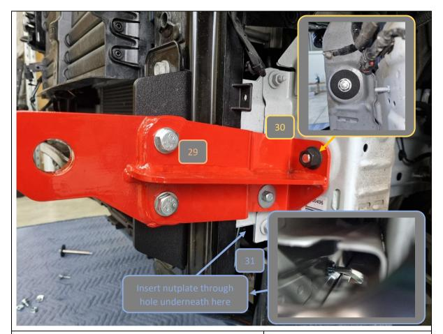
29. Loosely secure the recovery point to the Tow Hook Support Bracket with 2x M12x55mm hex bolts, flat washers and flange nuts.
