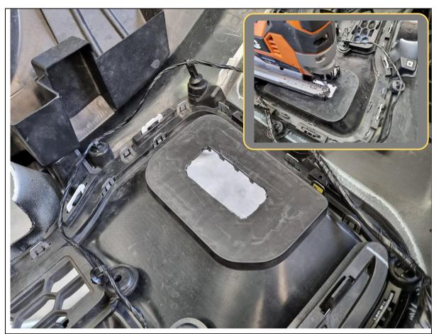
43. Using a jigsaw or similar tool, cut the bumper along the marked lines.
