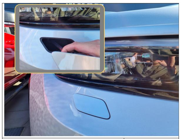
15. If headlight washers are equipped, pull out the plastic cover cap and unclip it from the plastic washer stem.
