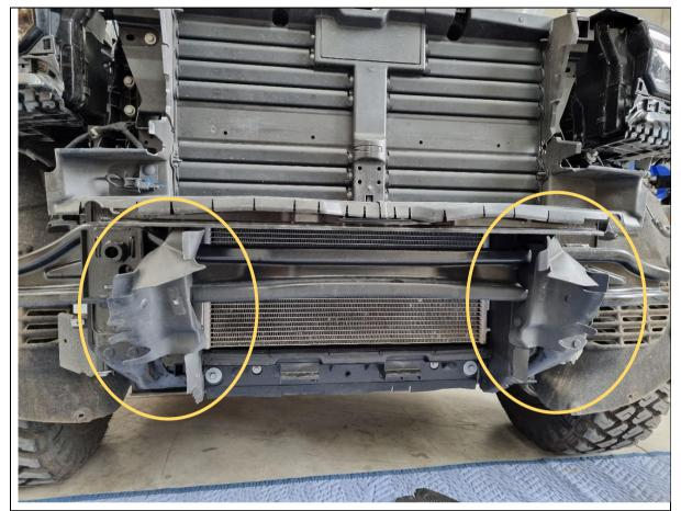
19. Unclip and remove the air dams with a flat head screwdriver or trim tool. Retain for reassembly.
