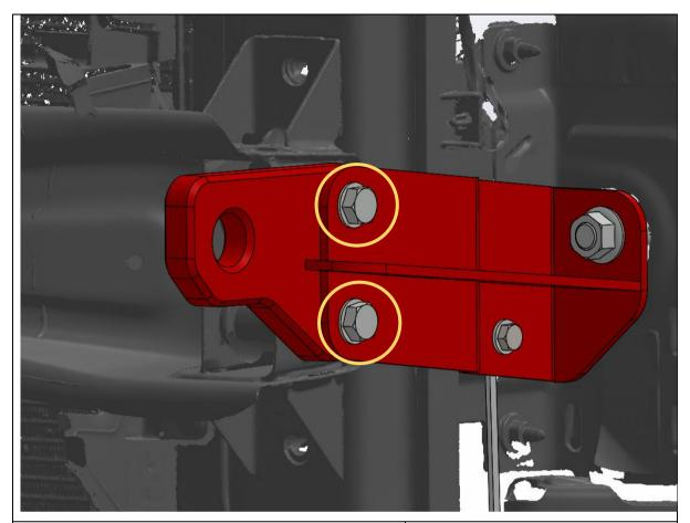
34. If your vehicle had an impact beam that did not require cutting, fit the recovery point to the impact beam with the factory tow hook fasteners.
